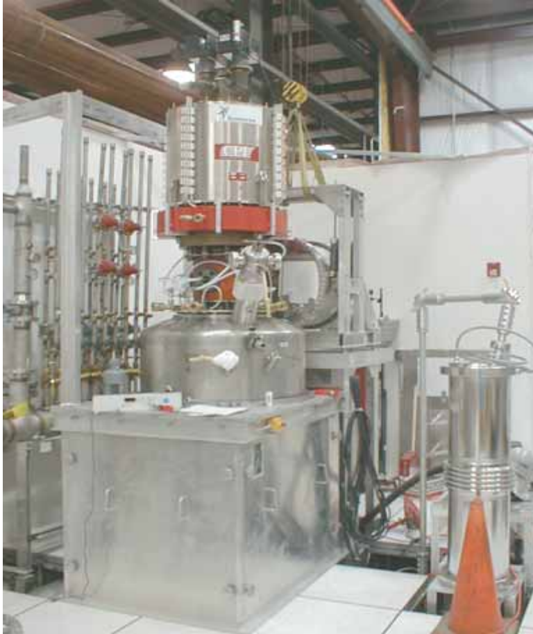
1 MW, 110 GHz Gyrotron at General Atomics
